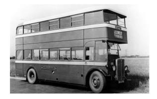
Left: A huge fleet of AEC Regents with Brush lowbridge bodies entered service with South Wales Transport in 1932. These operated over the longer routes, such as that to Brecon. The bodies were not Transport in 1932. These operated over the longer routes, such as that to Brecon. The bodies were not very durable and most were sold at an early stage. The bus uppermost [WN 4892] was fitted with an oil engine when two years old. [J. Higham]
