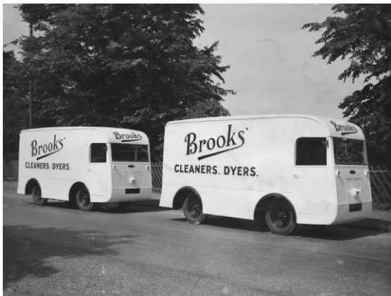
Two 'Morrisson-Electric' vans built to the 'National Standard' war time specification (refer text), and supplied new in June 1942. Note, not yet registered, and war-time blackout single headlight.
