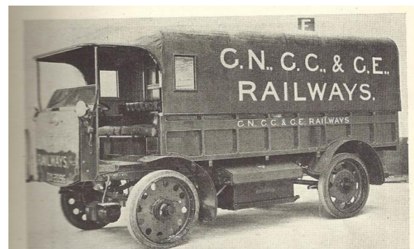
Fig. 2.—AN EARLY RANSOMES "ORWELL" VEHICLE Used for local deliveries by a railway company. The drive was on the front wheels.
