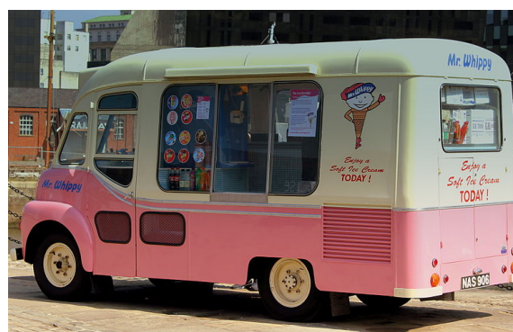
A typical Mr Whippy Karrier van. As a sister company to Commer, Karrier often manufactured brewers' drays or civic vehicles for the public sector. They used smaller wheels than their Commer counterparts to allow a lower cargo loading height or a lower body height to facilitate street cleaning. This example uses standard size wheels.
