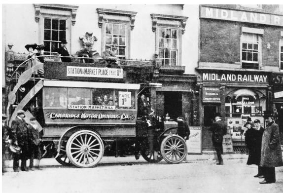
Above: The Midland Railway ran a bus feeder service between Cambridge station and the Market Place using the Cambridge Motor Omnibus Co as its contractor. Note the very early design of the wheels of this Thorneycroft, with their wooden spokes. The service started in April 1905 but by 1907 it had been taken over by the more successful Ortona, the services of which displaced the Cambridge horse tramway in 1914. [The Bus Archive]
