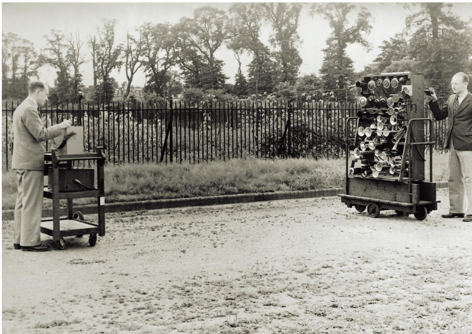
If ever a photograph deserved the full page treatment! Testing the acoustical properties of motor horns at the NPL in 1929 (Crown copyright)
