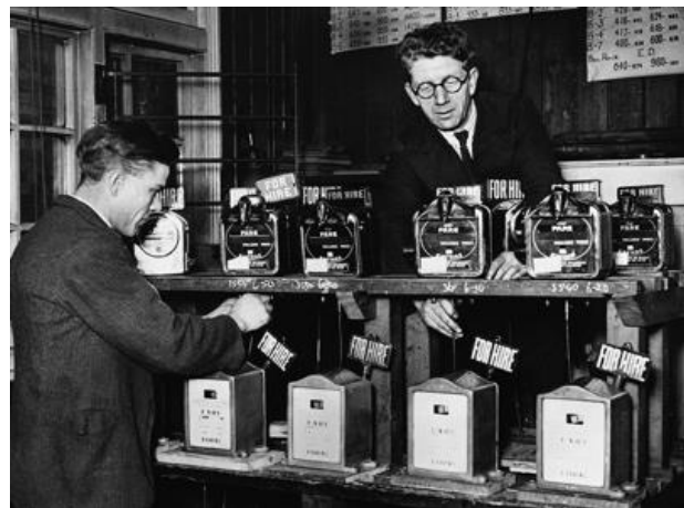
The taximeter test bench (crown copyright)
