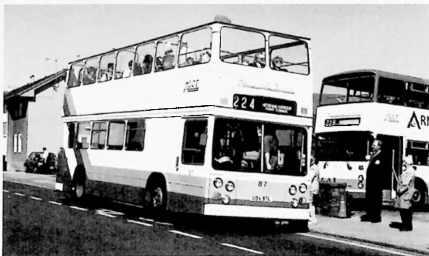
87 (UBV 87L) is an ex-Blackburn East Lanes bodied Leyland Atlantean that was converted to a high sided open topper for operation along Morecambe Promenade. The passengers on the well loaded upper deck patiently await a crew change outside the Depot.
