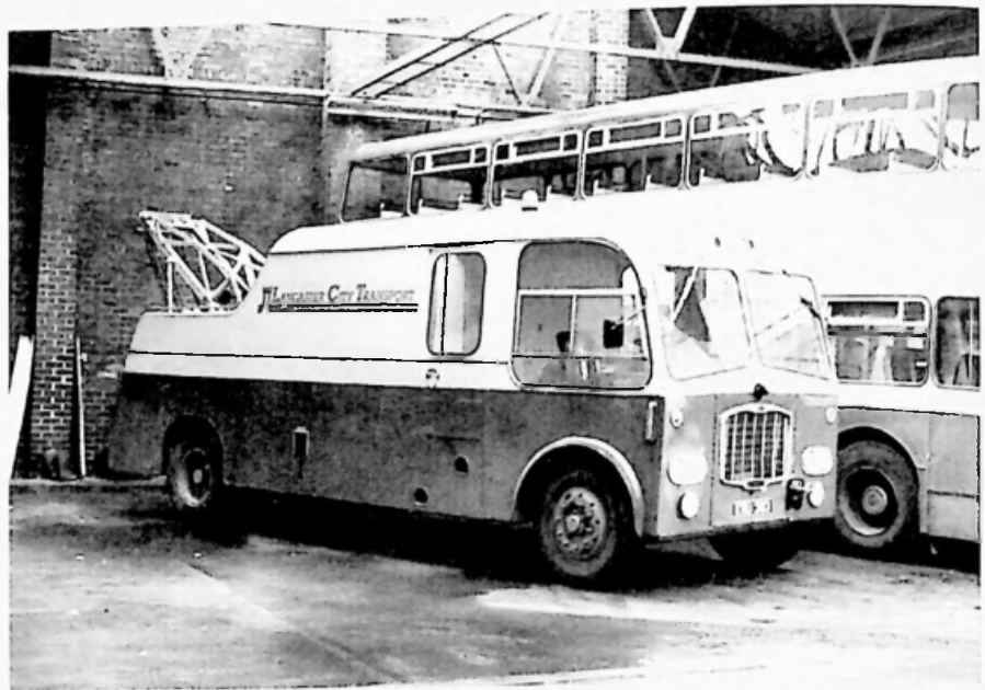
KWU 383 was an ex-West Yorkshire Road Car Bristol LWL6B that had earlier been fitted with a Gardner 6LW engine that suited LCT's needs for a breakdown vehicle. It had to be reregistered NSU 375 and is seen here in LCT's depot.
